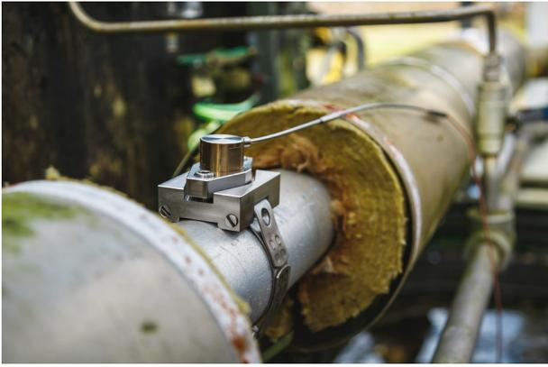
**Figure 2.** Low profile, high-temperature ultrasonic transducer for wall thickness and corrosion monitoring.
