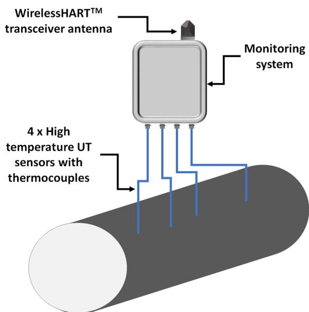
**Figure 1.** An idealised non-invasive UT monitoring system consisting of multiple high temperature capable UT sensors/transducers with integrated thermocouples connected to a separate WirelessHART™ enabled monitoring system. The monitoring system may be located in a convenient location for access.
