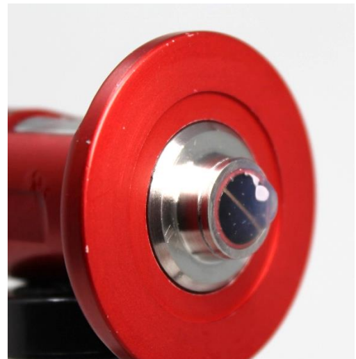
Apply couplant to the transducer face
