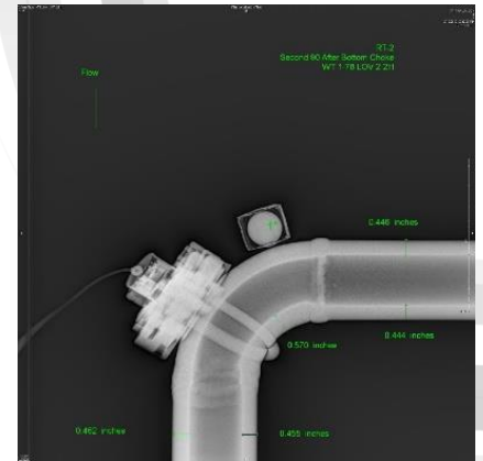
Figure 2: Example RT profile validation of the UT sensor measurements.
