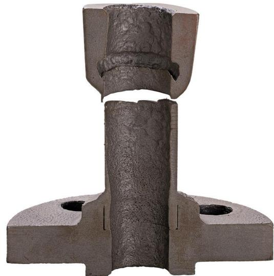
*Figure 1: High-temperature sulfidation corrosion of 12CrMo steel pipe (Photo by CEphoto, Uwe Aranas)*
