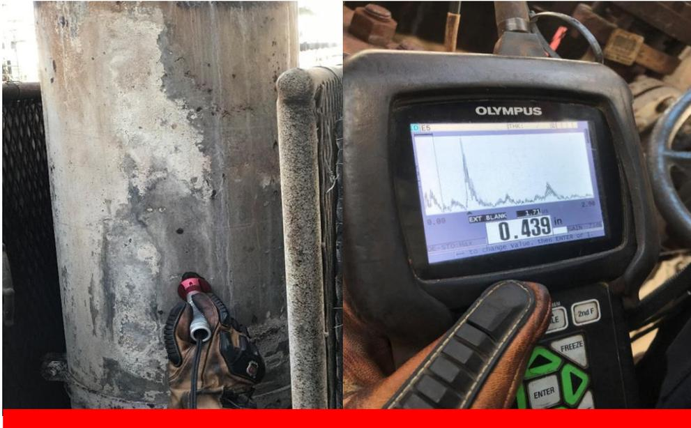
*Fig. 1 (Left) Ionix HS582i probe in use at US Oil Refinery by a Mistras Inspector. Pipe temperature readings at time of this inspection were 582°F (305°C). (Right) The thickness measurements were able to be repeated several times with minimal cool down periods.*
