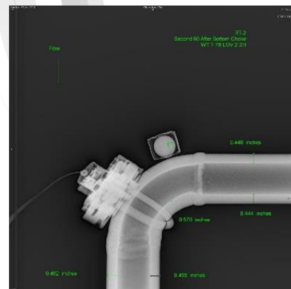
Figure 2: Example RT profile validation of the UT sensor measurements.
