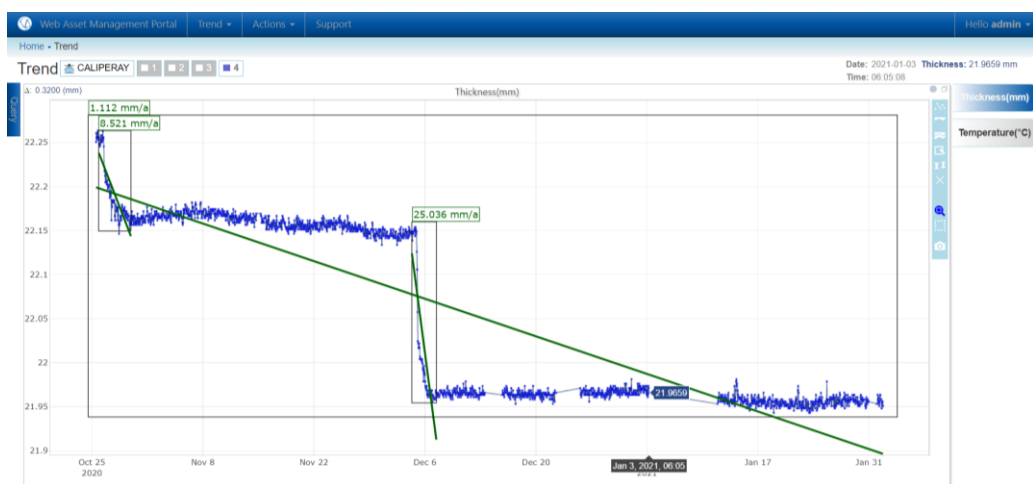
Figure 1: WAMP server analysis tool showing periods of accelerated wall loss on HotSense sensor 4.
