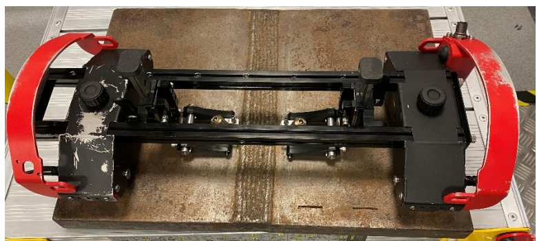
Figure 1: Photograph of the modified Lyncs scanner for high-temperature use on the test block.
