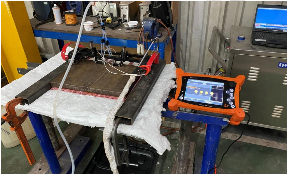
Figure 1: Photograph of the evaluation setup at Iris NDT (Immingham, UK)
