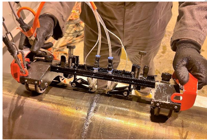
Figure 1: Photograph of the modified Lyncs scanner with probes for high temperature shown on a pipe section.
