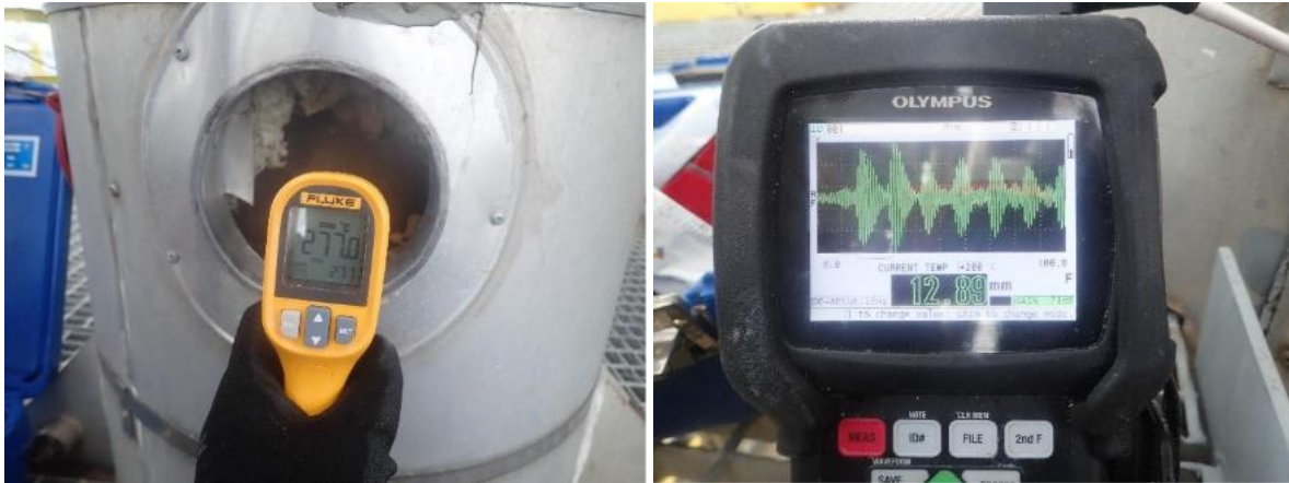
Figure 2: Lower frequency transducer allowed accurate, repeatable in-service inspection.
