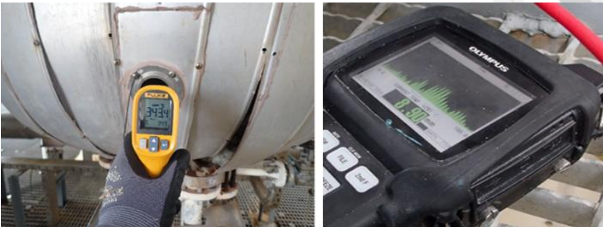
Figure 1: 5 MHz probe, producing an insufficient signal-to-noise ratio.
