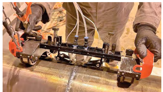
Figure 1: Photograph of the LYNCS HT scanner with probes for high temperature shown on a pipe section.
