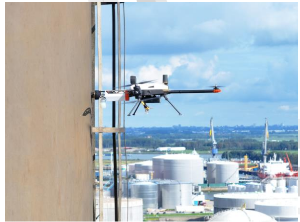
Fig. 1 Ionix HS582i probe in use on a Voliro T UAV platform
