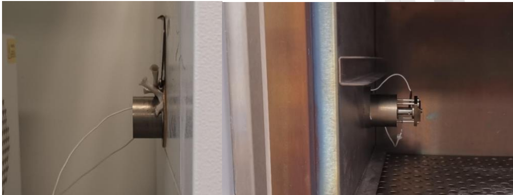
Figure 2 – Transducer and testing rod were placed inside an oven, with the bottom of the testing rod protruding through a port
