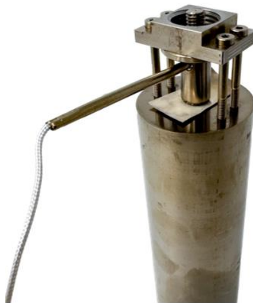
Figure 1 – Photograph of AE transducer coupled to a 200 mm length Ti rod
